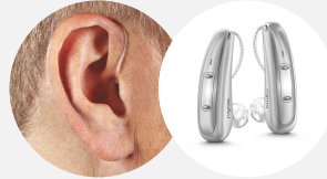
Receiver in Canal: Battery Operated
